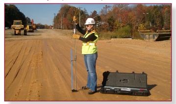
DCP Model K100AE is strong, compact and ergonomically designed for one person to use.
