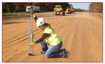
DCP Model K100DM is strong, compact and ergonomically designed for one person to use.
