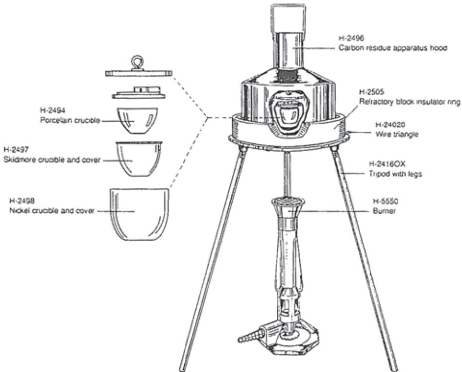
H-2495, Conradson Carbon Residue Apparatus
