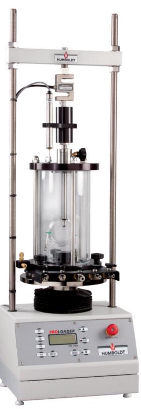
The HM-2900 ProLoader has been specifically designed to handle triaxial testing applications, including: UU, CU and CD triaxials, UC. From educational institutions and consulting firms to high-volume commercial labs and construction projects, the ProLoader can handle any application with ease. With its 3,000 lb. load capacity, the HM-2900 can easily handle all basic triaxial tests with ease.
